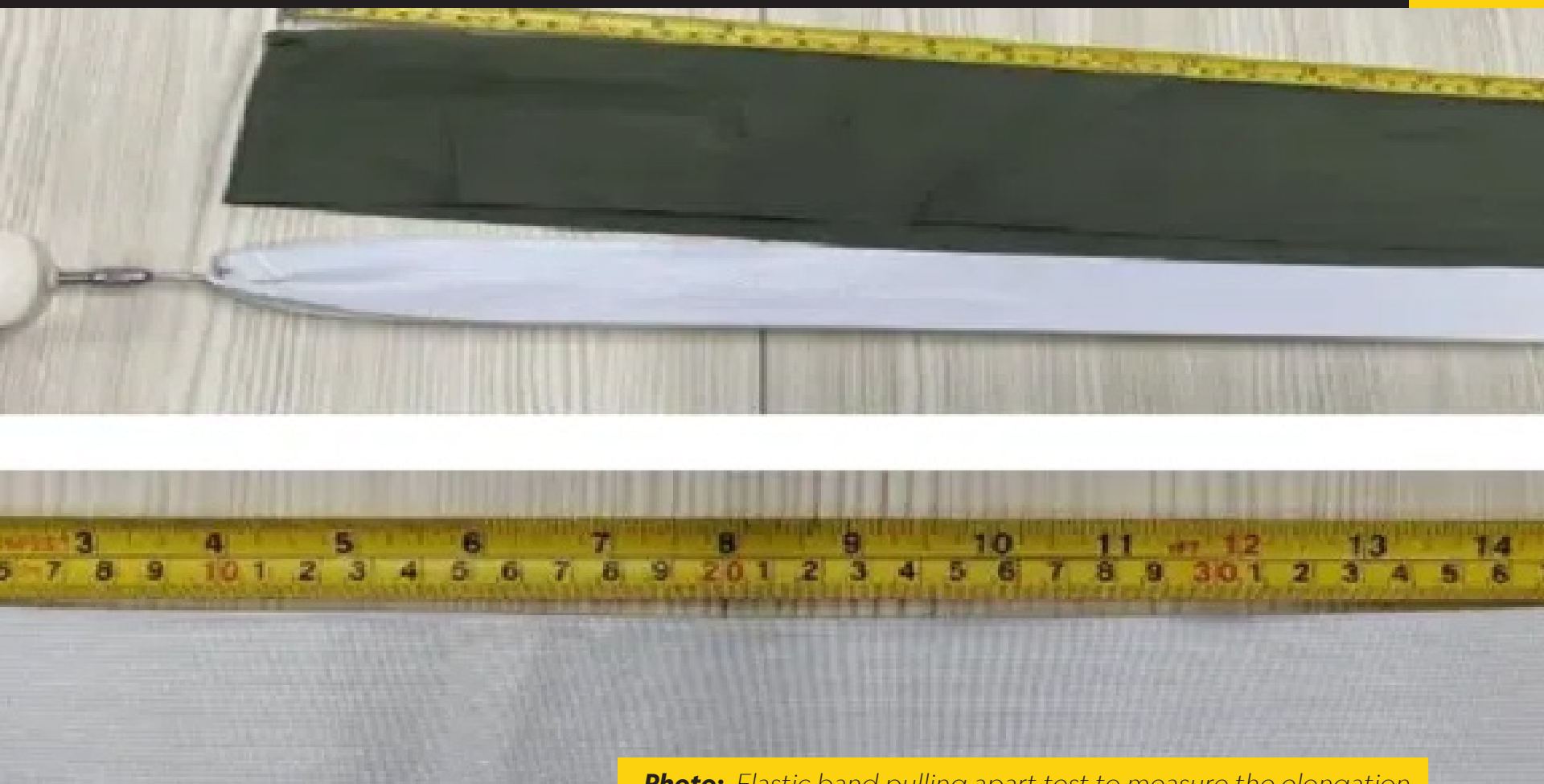
Photo: Elastic band pulling apart test to measure the elongation
